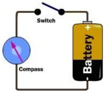
Let's say that you take another wire and place it parallel to the battery's wire but several inches (5 cm) away from it. If you connect a very sensitive voltmeter to the wire, then the following will happen: Every time you connect or disconnect the first wire from the battery, you will sense a very small voltage and current in the second wire; any changing magnetic field can induce an electric field in a conductor -- this is the basic principle behind any electrical generator. So:
