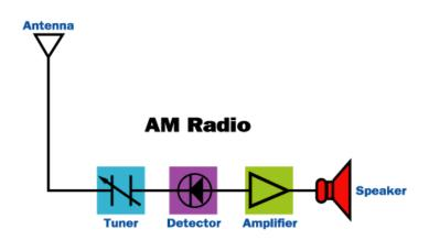
Unless you are sitting right beside the transmitter, your radio receiver needs an **antenna** to help it pick the transmitter's radio waves out of the air. An AM antenna is simply a wire or a metal stick that increases the amount of metal the transmitter's waves can interact with.
