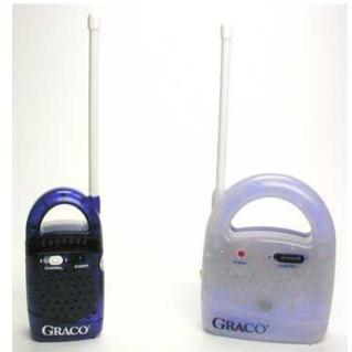
A typical baby monitor, with the receiver on the left and the transmitter on the right: The transmitter sits in the baby's room and is essentially a mini "radio station." The parents carry the receiver around the house to listen to the baby. Typical transmission distance is limited to about 200 feet (61 m).
