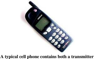
A typical cell phone contains both a transmitter and a receiver, and both operate simultaneously on different frequencies. A cell phone communicates with a cell phone tower and can transmit 2 or 3 miles (3-5 km).
