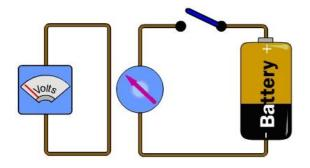
One important thing to notice is that electrons flow in the second wire only when you connect or disconnect the battery. A magnetic field does not cause electrons to flow in a wire unless the magnetic field is **changing**. Connecting and disconnecting the battery changes the magnetic field (connecting the battery to the wire creates the magnetic field, while disconnecting collapses the field), so electrons flow in the second wire at those two moments.
