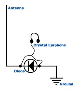
Now if you put the earplug in your ear, you will hear the radio station -- that is the simplest possible radio receiver! This super-simple project will not work if you are very far from the station, but it does demonstrate how simple a radio receiver can be.
